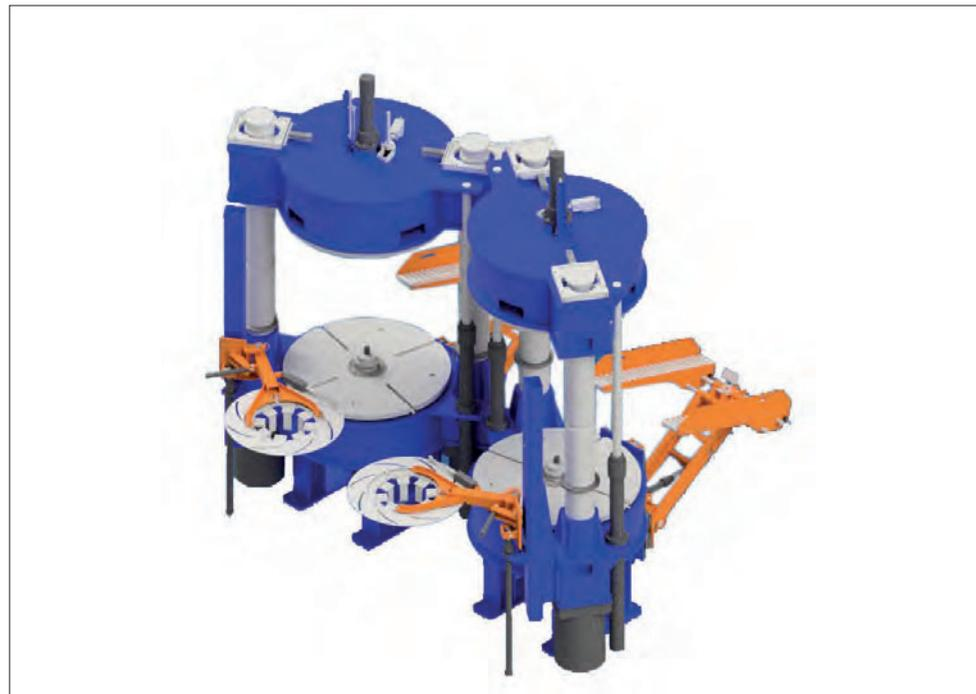
Therefore, the press does not need multiple locking points and can work perfectly well with just one. Columns rise at the end of each cycle and release the locking plates from grooves, meaning the locking mechanism can work without jamming.
