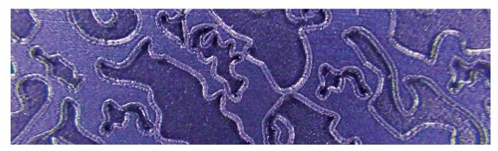
aser engraving is one of the latest trends in the tire molding business. This methodology enables users to engrave very small details with traditional machining processes, which is not normally possible. The technology is not powerful enough to replace CNC methodology yet, however, and is also limited by the fact that there is a requirement for larger surfaces, but it is currently suitable for use in many situations in tire production, useful for both tire manufacturers and mold makers.
